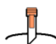
Extend standpipe into the vessel and cut the end at a 45° angle.
