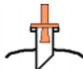
Extend standpipe into the vessel and cut the end at a 45° angle.
