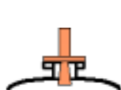
Use a shorter standoff so end of transducer assembly is inside vessel, or...
