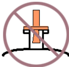
Do not mount end of transducer assembly inside standpipe.
